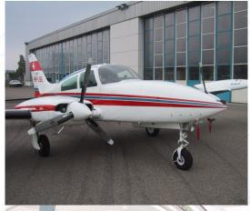
The Cessna 310 is a twin engine airplane, powered by two turbo charged piston engines. The cabin is not pressurized and it offers place for up to five passengers in a economy way of seating.
